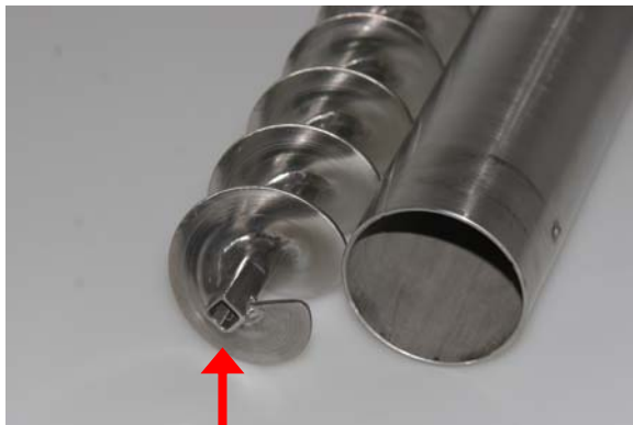
Square Receptacle Auger Photo 9.3
